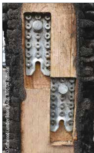
RICON'S connector after 90 minutes and MEGANT® connector after 60 minutes fire tests. The wood is charred all around. The connectors withstood the vertical load applied in the fire test.
