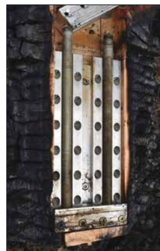
RICON'S connector after 90 minutes and MEGANT® connector after 60 minutes fire tests. The wood is charred all around. The connectors withstood the vertical load applied in the fire test.
