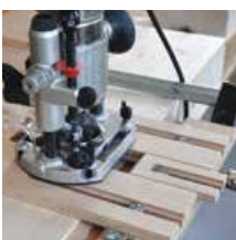
Mill with with routing-jig
