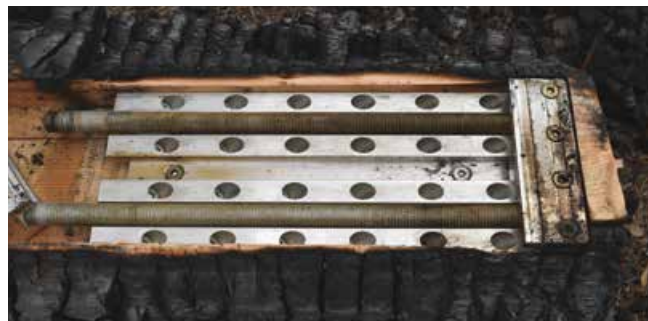
MEGANT® connector after 60 minutes fire test. The wood is charred on all sides. The connector withstood the applied vertical load in the fire test.
